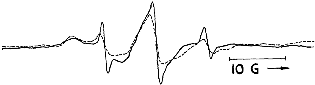
Figure 6. Long-term reduction of spin labels. —, soluble oxidase, 1 h after addition of reducing system; ----, same solution, 21 h later (gain is 20× higher).
